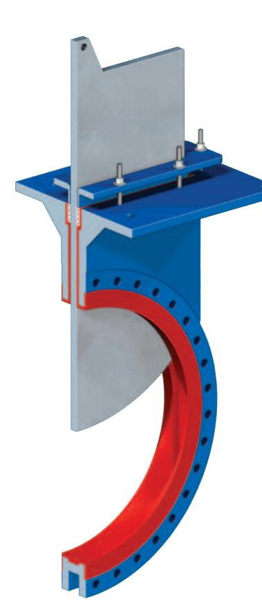
The Fabri-Valve® S16-ULV Urethane Lined Knife Gate Valve provides an economical solution for abrasive and corrosive applications requiring large diameter valves. The S16-ULV utilizes ITT's perimeter sealing technology that has been utilized for over 20 years. The S16-ULV features a robust perimeter sealing design that provides a no-discharge, bi-directional, drip tight shutoff.
